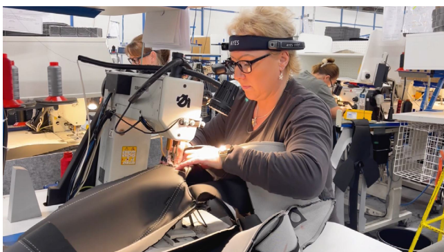
The display of the glasses shows individual workflows, guiding the worker step by step to complete them.
